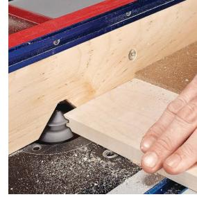
▲ Face Down. Rout the first part of the joint with the inside face of the workpiece down on the router table. A backer board prevents tearout.
