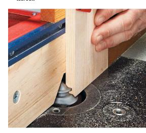
On End. The mating part of the joint is cut with the workpiece held vertically against the fence. The backer board helps keep it square.
