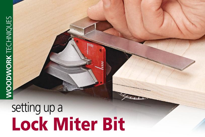
A handy gauge takes the hassle out of setting up this versatile bit in your router table.
