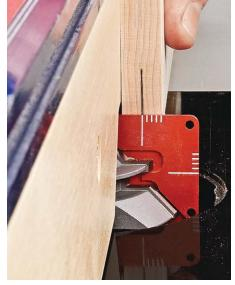
Fence Setting. With the part held vertically, move the fence until the centerlines meet.
