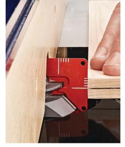
▲ **Bit Height.** Raise the bit so the line on the gauge aligns with the one on the workpiece.
