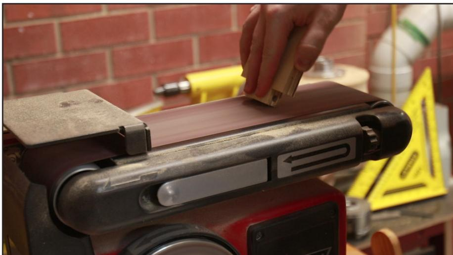
Separate the two parts out, and take them to a sander (or router table with roundover or bullnose bits) and sand a curve into it so the hinge can actually pivot
