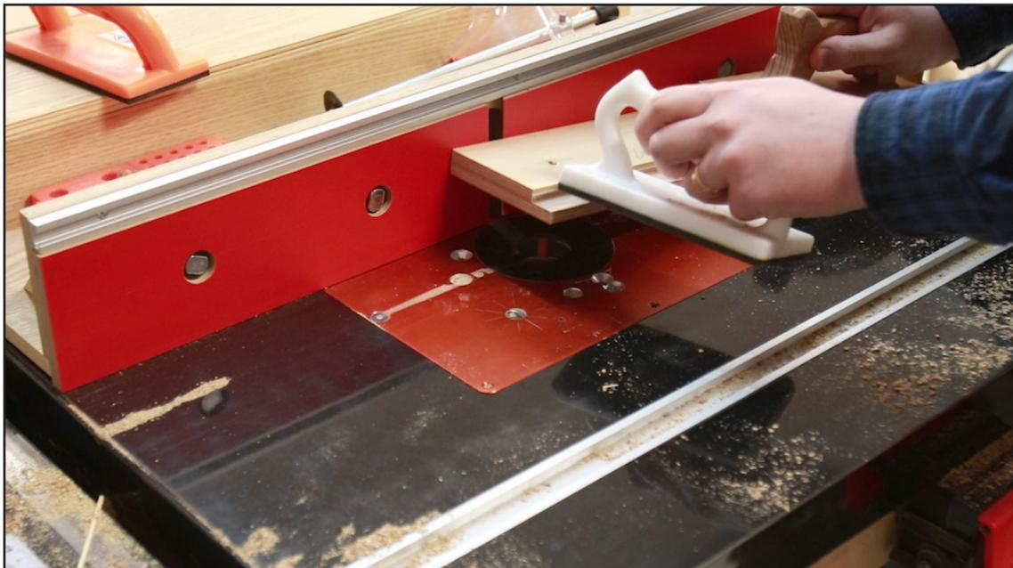
Using the same 5/16” router bit from earlier, over at the router table “connect-the-dots” and route the groove between the two previously drilled holes. Do this in stages of about 4mm height per pass. Cut the remaining T-Track down to 500mm and mount it to the groove in the aux fence.
