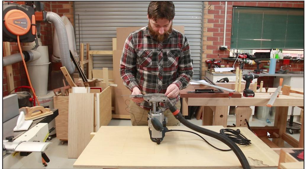
Using the 1/2" cutter first, route a groove slightly deeper than the thickness of the T-Track bolts. If the bolt head is proud, it'll drag on the table saw surface and skew the sled. At the "back end" (towards the back fence) of the sled, plunge all the way through the material to create a cut out large enough for the bolt head to pass through. This slot should be about 25mm long.
