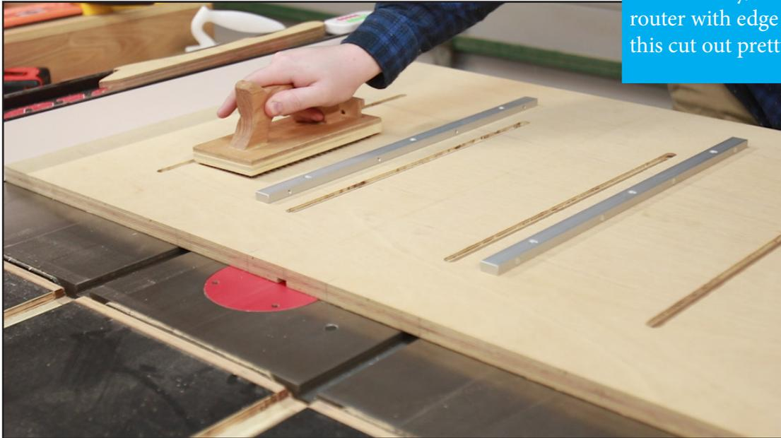
Alternatively, a router table or router with edge guide can make this cut out pretty easily.
